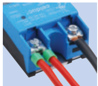
Direct connection by wire or tip 2 x 6 mm 2 (AWG10) fine strand i.e. 32A 2 x 10 mm 2 (AWG8) solid i.e. 50A
