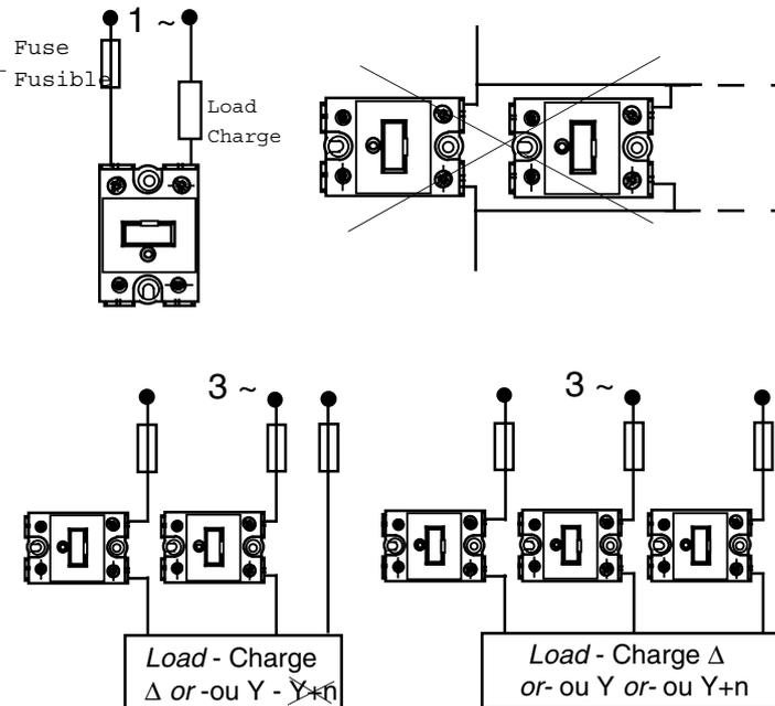
⚠ Must be used only in conjunction with a heatsink mounted in vertical position to help the air flow. Minimum air distances all around the heatsink : 10mm.
