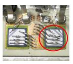
The typical failure for the celduc SSRs was a lift-up: which means that the bonding wire is no longer connected to the power chip. This is due to its small size and flexibility. With this type of failure you have less risk of fire as it results in an open-circuit.
