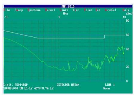
You can find standard « low noise » SSR on the market but those are limited to low switching current of 5A for domestic applications or to low inductive loads, while lots of pure resistive loads applications have high emission noise.
