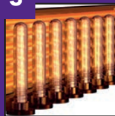
Re-heat station by infra red heating lamps
