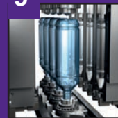
Stretch Blow Molding with hot air
