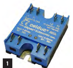
Two-phase SOB SSR to control heating elements wired in a delta connection. Specifically designed for high voltage loads, balanced or not.
