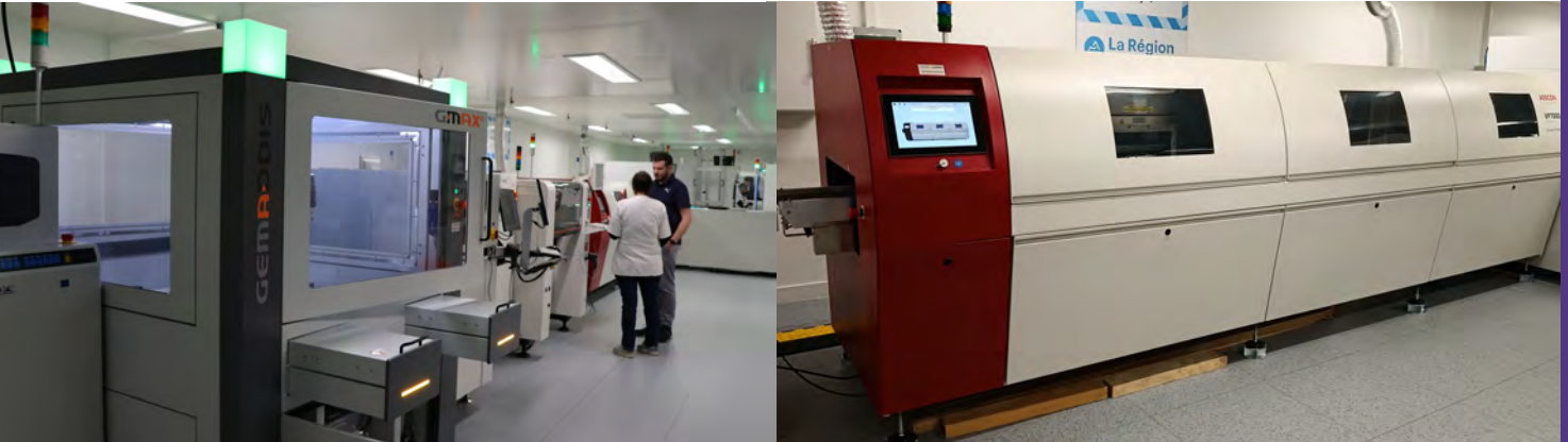
Four-phase vapor reflow oven with vacuum and cooling
